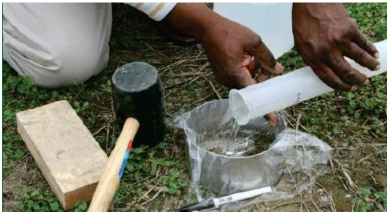
Figure 8. Water is poured into the plastic-lined tube.
